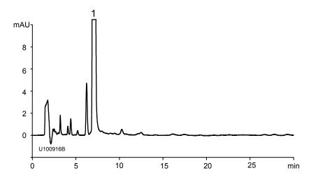
Column : YMC-Triart C18 (5 μm, 12 nm)
