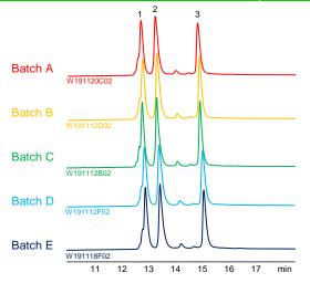
Column : BioPro HIC HT 2.3 µm, 100 X 4.6 mml.D. A) 100 mM NaH<sub>2</sub>PO<sub>4</sub>-Na<sub>2</sub>HPO<sub>4</sub> (pH 7.0) containing 2.0 M (NH<sub>4</sub>)<sub>2</sub>SO<sub>4</sub> Eluent
