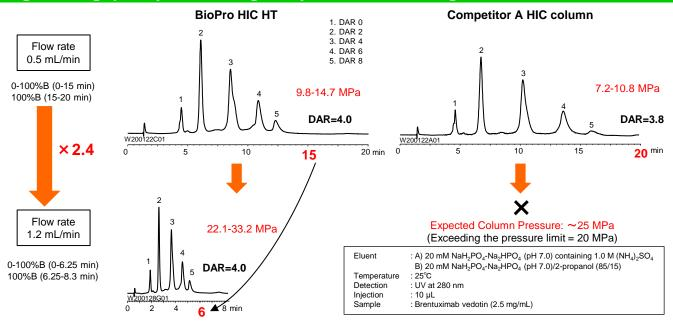
BioPro HIC HT consists of the fine non-porous polymer particle designed for separation of proteins, and has high pressure tolerance with excellent chromatographic resolution by optimized packing condition. This is capable of the rapid analysis without losing the resolution at a high pressure, which is too high to use with the other commercially available HIC column.
