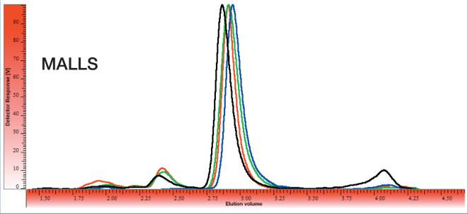
Figure 1: Chromatograms of Avastin® using different eluents. Top: UV at 280 nm. Bottom: MALLS detection trace (90° angle).
