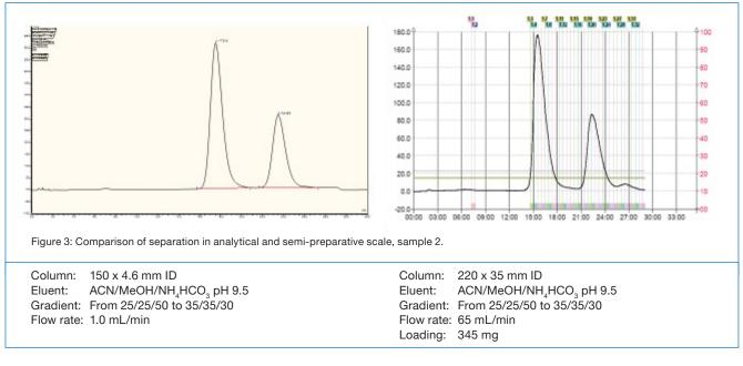
This easy method transfer was demonstrated using an alternative sample. Again, the approach showed successful results. Even with a loading of 345 mg, an efficient separation was achieved.
