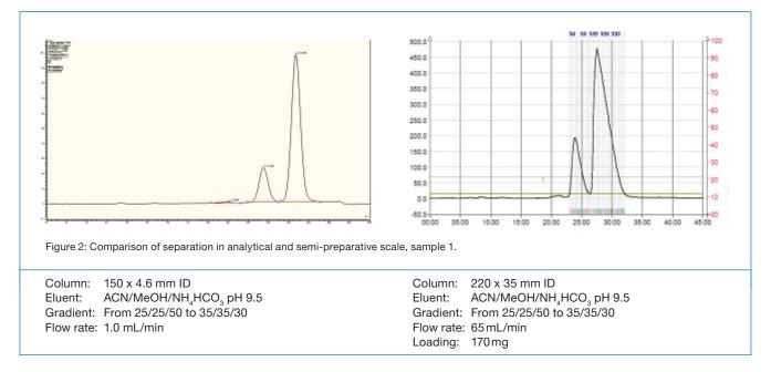
The results in Figure 2 show that the method can easily be transferred from analytical to semi-preparative scale. Due to the same packing quality in the pre-packed glass column, the same separation could be achieved with a loading of 170 mg and a flow rate of 65 mL/min.
