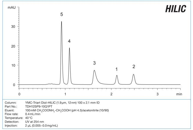
Figure 3: Separation of the five markers using a YMC-Triart Diol-HILIC UHPLC column.
