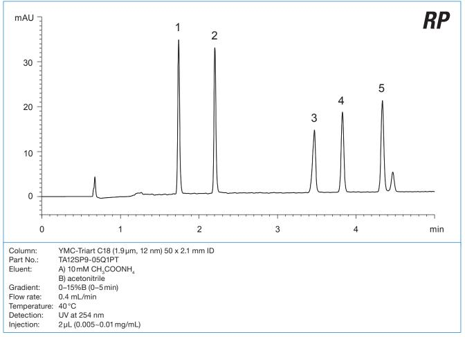
Figure 2: Separation of the five markers using a YMC-Triart C18 UHPLC column.
