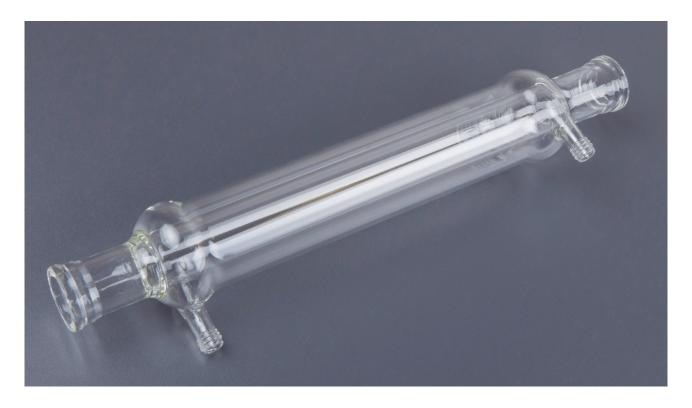
Borosilicate glass 3.3 heating jacket provides full organic solvent compatibility for efficient cleaning. This can drastically extend the column lifetime.
